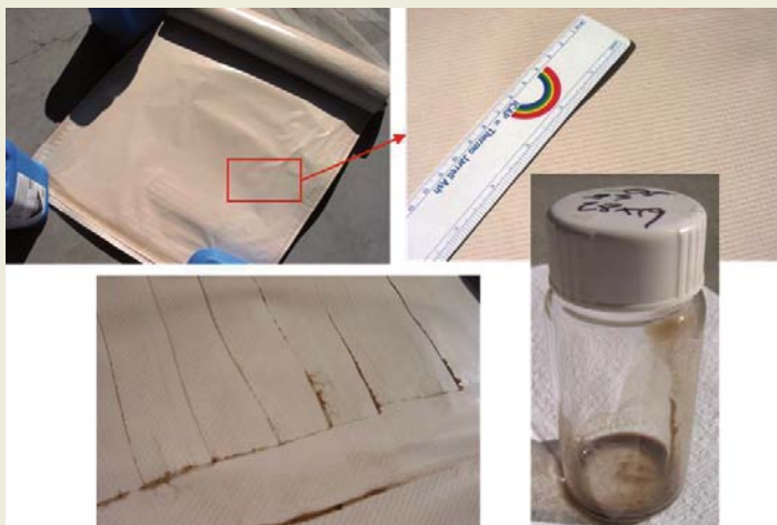
Figure 5 Images of a third-stage RO element removed for autopsy.
